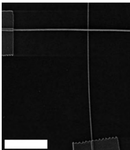
Figure 1. SEM image of a crossed nanowire device assembled from a CdS nanowire (horizontal) and a silicon nanowire (vertical). Scale bar: 2 \mu\text{m} .
